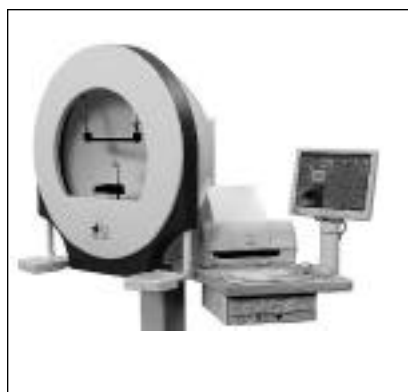
Fig. 1 - Experimental design: twinfield-perimeter with test bowl, computer monitor, personal computer, and printer.
